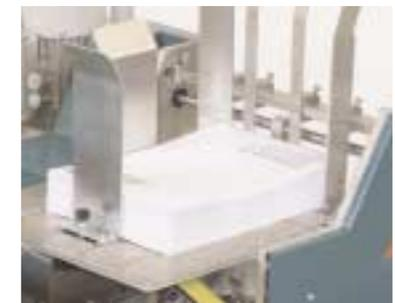
The envelope station is based on the same rotary technology as the insert feeders
