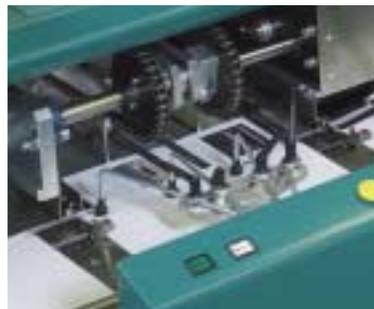
The insert into envelopes - based on tried and tested technology - manages the load and strains of continuous high speeds. The envelope-table briefly stops by the insert and inserts are guided into the envelope.
